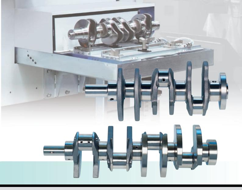
The HL 1000 is designed to machine crankshafts of up to 1000 mm length and 265 mm diameter. With bore diameters of between 4 and 8 mm and the use of minimum quantity lubrication, the HL 1000 achieves the kind of tool life that is far beyond the usual. Finally, all machining results – even those for truck crankshafts weighing up to 150 kg – are checked and logged by the control system while the workpiece is still clamped. The machine base is of Mineralit<sup>®</sup> (reaction resin poly-
