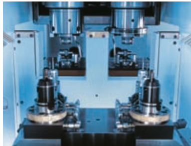
VSC TWIN Series Vertical multi-spindle machine, simultane- ous machining of 2 chucked components
